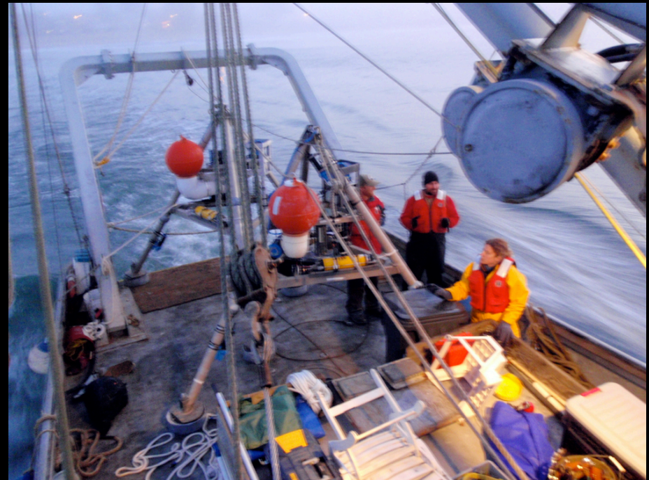
Deployment of hydrodynamic and sediment transport tripods from the R/V Shana Rae
